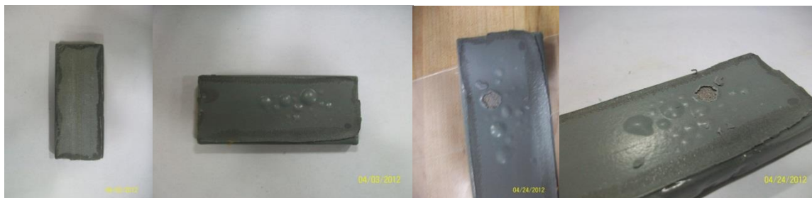
Madison Chemical Industries Failed Week 1 CorroPipe 3000 AM (Polyurethane)
