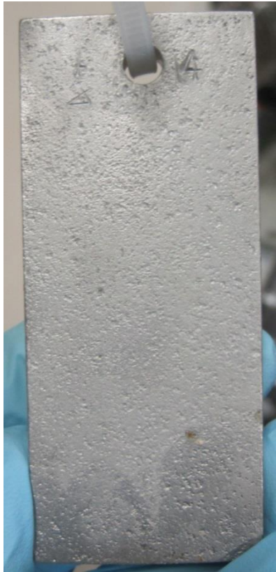
Control – In lab air, outside of process tank
