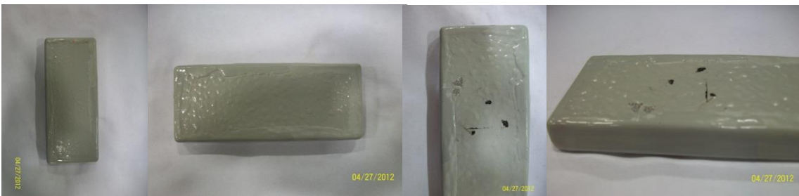
Tnemec Failed Week 5 Series F061 (Cycloaliphatic Amine Epoxy)
