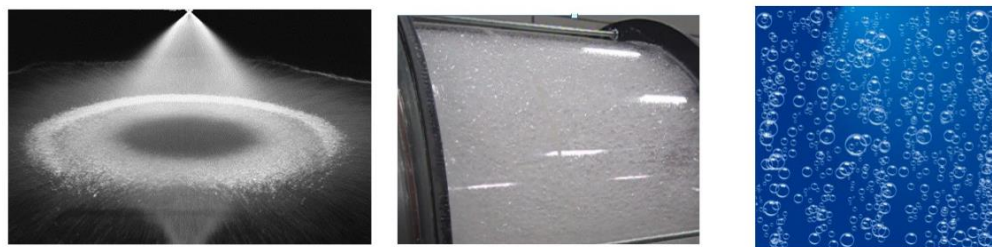
Fig. 2. Comparison of three methods for creating large contact area between a liquid and a gas: spraying, foaming, and bubbling.
