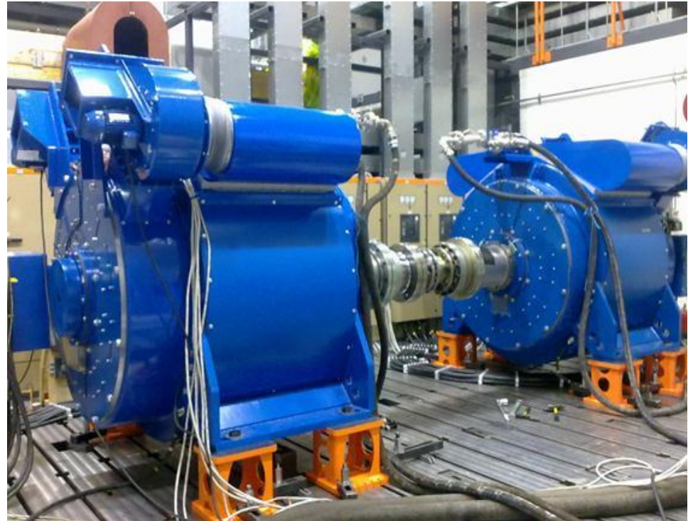
SustainX units undergoing back-to-back test
