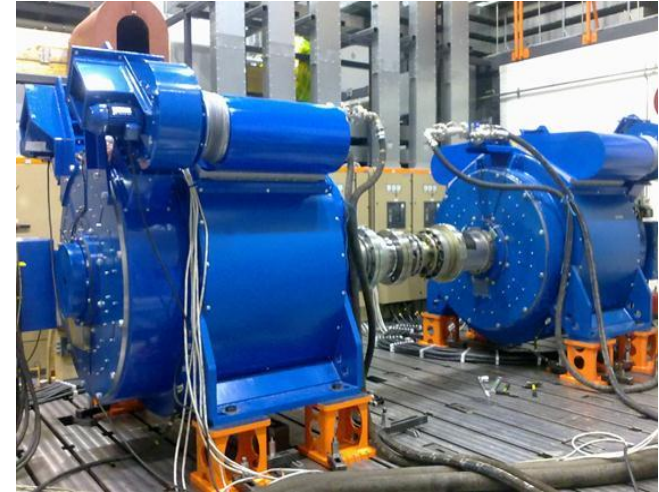
PERMANENT MAGNET GENERATORS
